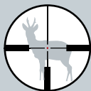
Reticle in the front (1 st ) focal plane
