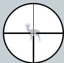
Reticle in the front (1 st ) focal plane
