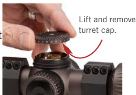
3. Re-install the cap, turning so that the "0" mark aligns with the reference dot on the turret body.
