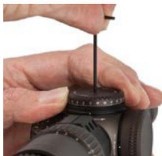
4. Re-tighten the central screw while holding the turret cap firmly between thumb and forefinger to prevent rotation.
