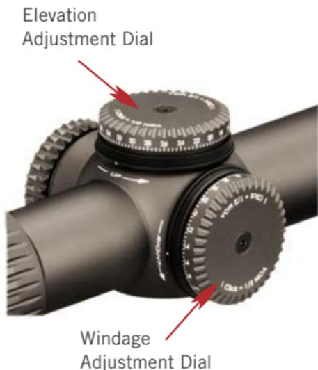
The Razor HD 1–6x24 riflescope uses clicks scaled in 1/2 minute of angle measurements (MOAs) so each small click will move the point of impact 1/2 MOA.
