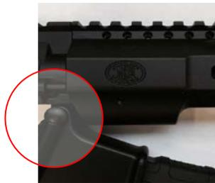
When dis-assembling the rifle as explained in Section 18.1, use extra care when separating the upper and lower receivers. Because of the mounting device on the rail, there is less clearance between the rail and the lower receiver. If the upper receiver is pivoted on the front take-down pin as shown in Figure 20 of the Owner's Manual, the rail may come in contact with the lower receiver causing damage to the rail, the lower receiver and potentially pinching your hand. Please use caution.
