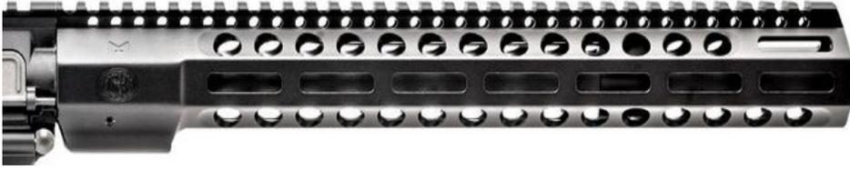
The FN Wedge Lock Rail Assembly 14.625" light weight free-float forearm/rail is installed on the FN 15™ DMR II in place of the standard round handguards. The wedge lock rail assembly extends over a low profile gas block. It allows for mounting of additional grips, sights, laser devices and other accessories onto a rigid, free-float forearm. Additional M-LOK™ slots fill the rest of the top rail.
